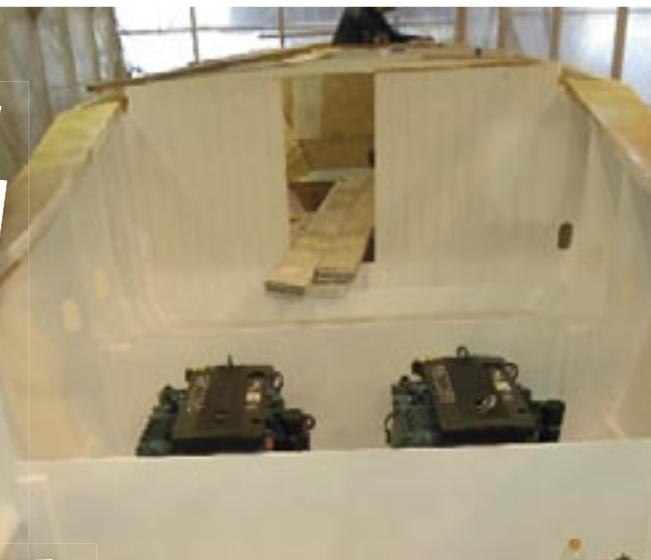
The boat is turned over inch by inch, resting it on the ground while straps attached to a crane are adjusted (1) around the hull. The inside panelling is installed before being coated in epoxy and painted. Then the fuel and water tanks are installed (2), as well as the two Volvo engines, with shafts and P-brackets fitted through the hull – all done by the yard team.
