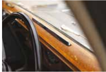
The chrome vents for the R Type's windscreen demister move to direct the flow of air
