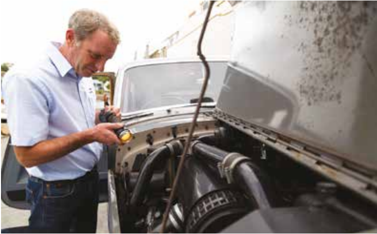
The 'fail-able' parts in the R Type's engine, such as the coil condenser and points, are doubled up – a technique Dave uses in boat building
