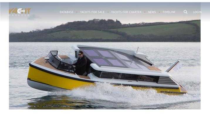
T/T Scout is operated via joystick control from the helm, accompanied with a reversing camera and bow thruster. Power comes from two Volvo D3 220 HP engines for a top speed of 37 knots.
