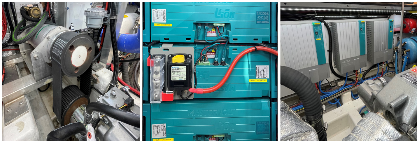
Above, L to R: Electric engine and drive belt connected to the prop shaft; Lithium-ion batteries; The inverters
