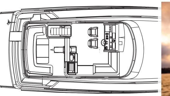
A popular option on the Hardy 50DS is the incorporation of a spacious flybridge, complete with an exterior helm (which mirrors the main helm), an outdoor galley and an abundance of seating for dining al fresco and entertaining with a view.
